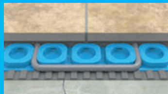
UNCOUPLING / CRACK ISOLATION
